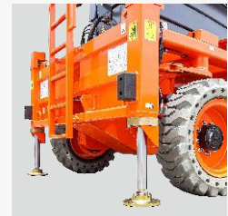
Automatic Leveling Outriggers
